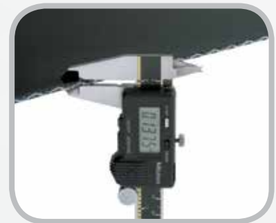
Measure belt thickness.
